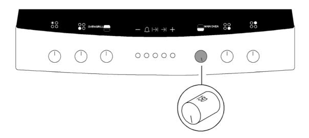
Turn the main oven temperature control to the required setting.
